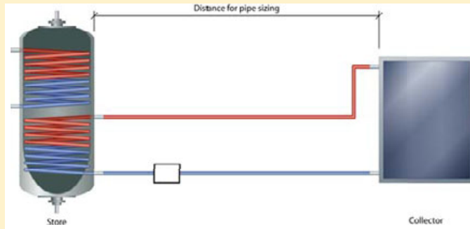
Figure 56 – Pipe Sizing distance
